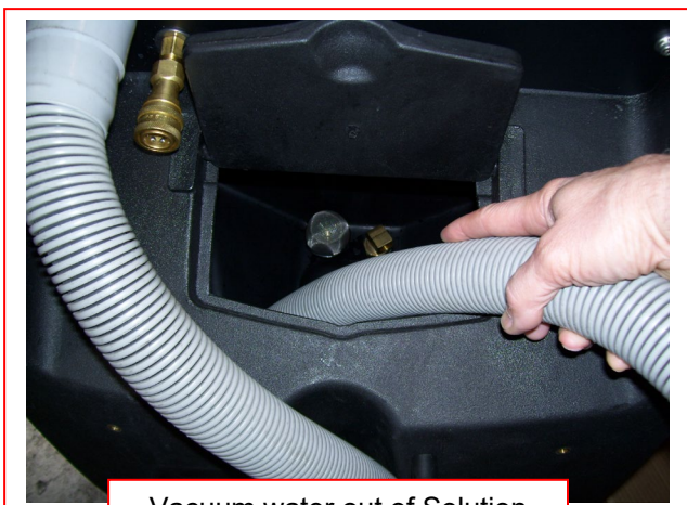
Vacuum water out of Solution Tank
